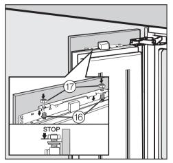
Open the door and hang the custom door with the mounting frame over the threaded bolts (6).
